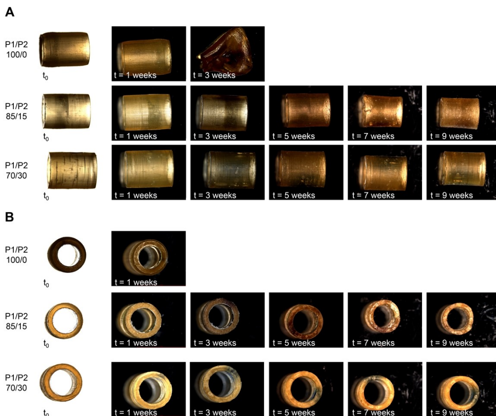
Figure S7. Changes in dimensions and surface morphology during the degradation study. Photographs of representative tubular objects based on P1/P2 100/0, 85/15 and 70/30, w/w at different time points. (A) Side view. (B) Top view.
