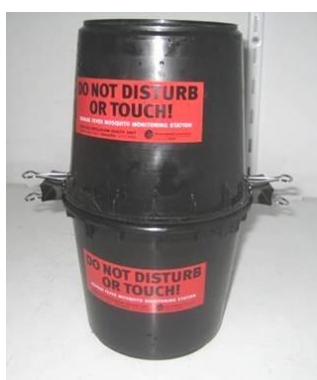
Fig. 5 (A). Clippy Trap showing the position of the bulldog fold back clips. (B) Top half of Clippy Trap showing glue panel due for replacement.
