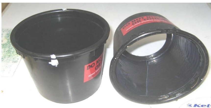
Fig. 4. The two halves of a Clippy Trap. Clip attachment points indicated by white marks (LHS bucket); glue panel held in place by Sika-Flex ridge (RHS bucket).
