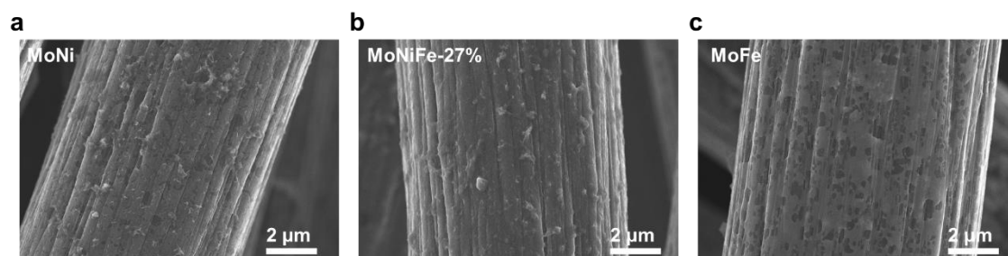
Supplementary Fig. 6. Morphology characterizations of MoNiFe (oxy)hydroxide.
