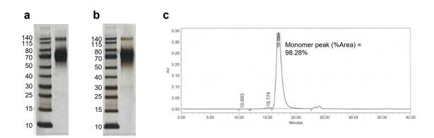
Supplementary Figure 1. SDS-PAGE and chromatography results for purified gE protein. (a, b) The purity of recombinant VZV gE protein was verified using SDS-PAGE followed by silver staining. SDS-PAGE was performed under (a) non-reducing and (b) reducing conditions. (c) The purity of the recombinant VZV gE protein was verified by size exclusion chromatography using a BioSep-SEC-s3000 column.
