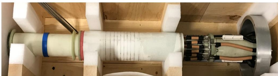
Figure S6. Custom-built MRI propulsion gradient coil. MRI combined propulsion and imaging coil developed in collaboration with Tesla Engineering Ltd. The coil is 786 mm in length, with an internal diameter of 60 mm, designed to fit a 9.4 T Varian Inova MRI scanner. Magnetic field gradients of up to 1150 \text{ mT m}^{-1} can be achieved along all three axes, when driven by 200A, 350 V amplifiers, with rise times of no more than 21 \mu\text{s} .
