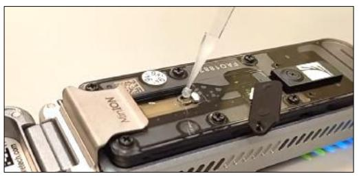
Close the SpotON port and the Priming port cover. The flow cell is now ready for sequencing.
