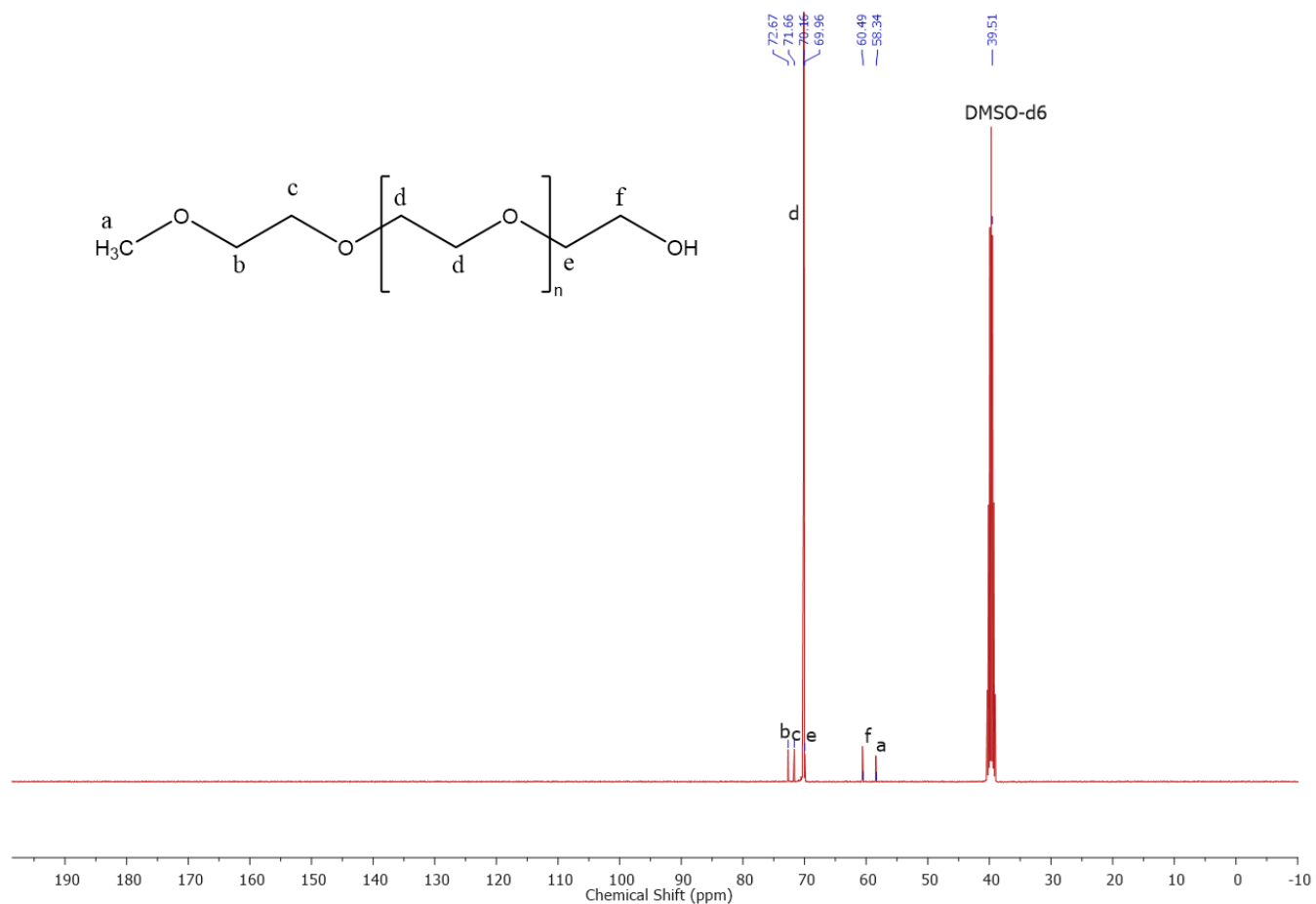
Figure S5. ^{13}\text{C} NMR spectrum of mPEG 2000 in DMSO-d 6 , recorded on Bruker AV-500 NMR.
