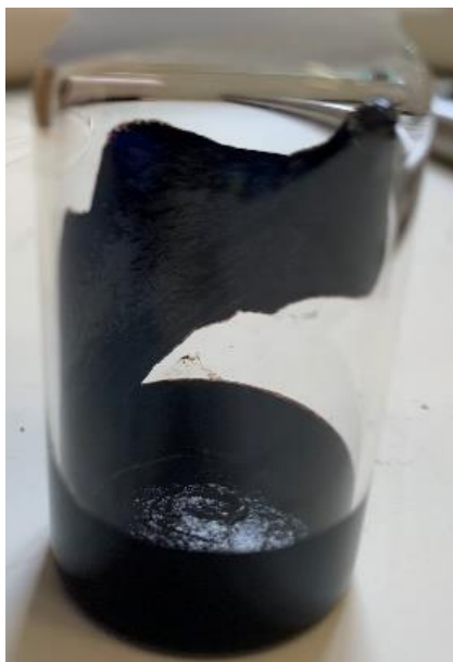
Fig. S2. CNT dissolved in oleum at high concentration. 5 mg of CNTs dissolved in 0.5 mL of oleum.
