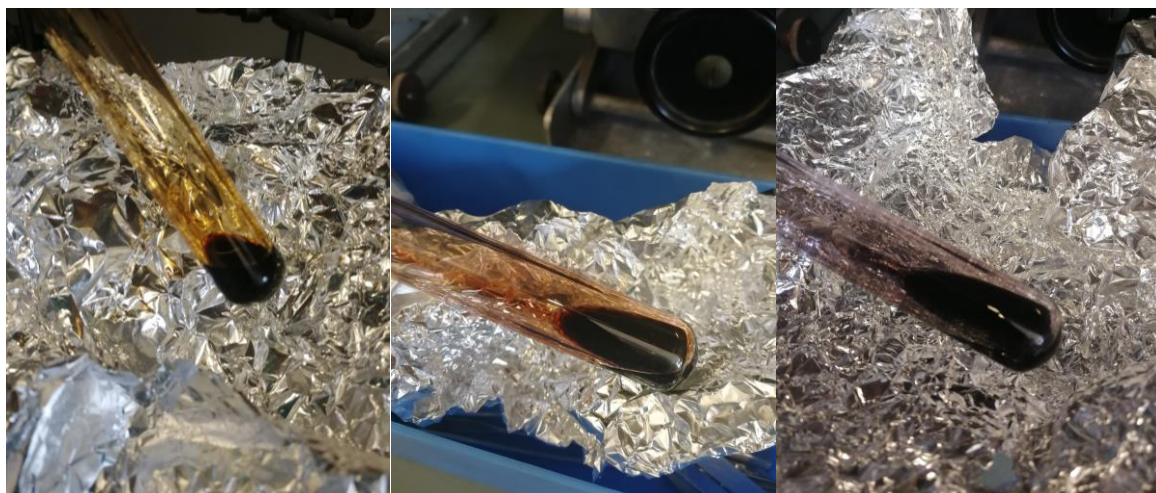
Fig. S10. Solution of \text{Cp}^*_2\text{Co} in DMA under \text{N}_2\text{O} . ( left , t = 2 min; middle , t = 10 min; right , t = 90 min).
