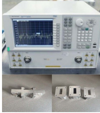
Fig. S9 Experiment setup for EMI shielding measurement: vector network analyzer.
