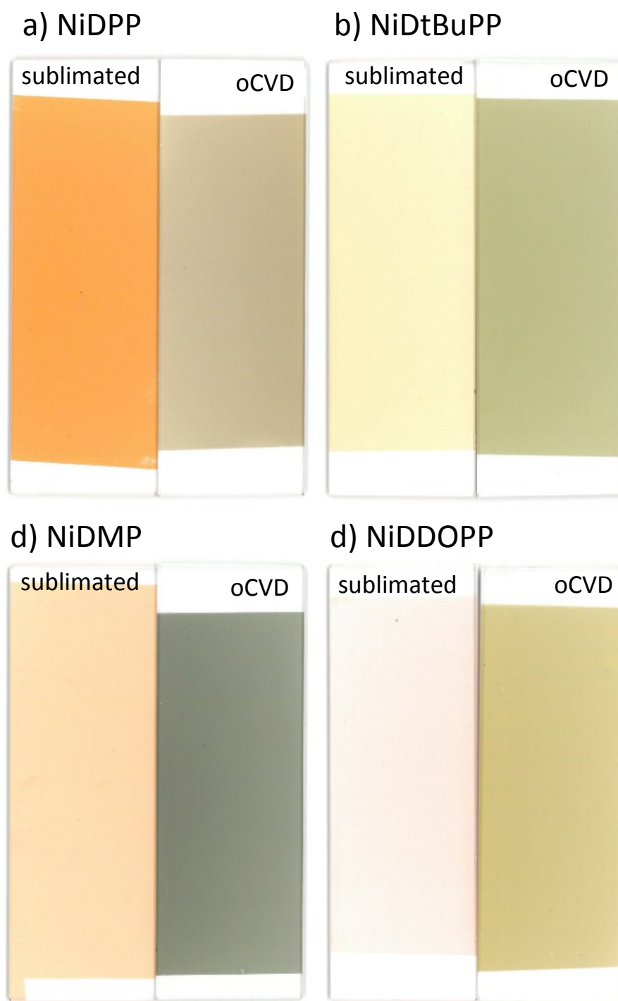
Figure S4. Optical image of the different coating obtained by simple sublimation (left) and oCVD (right) for each porphyrin on microscope glass. a) NiDPP, b) NiDtBuPP, c) NiDMP and d) NiDDOPP.
