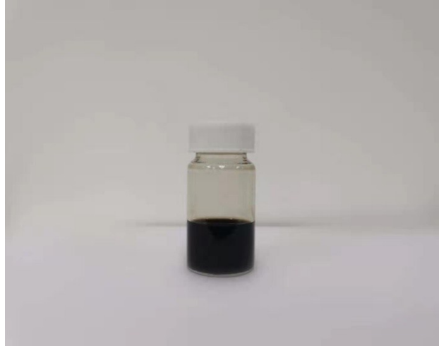
Figure S2. Photograph of the GNRs ink showing good dispersity in water.
