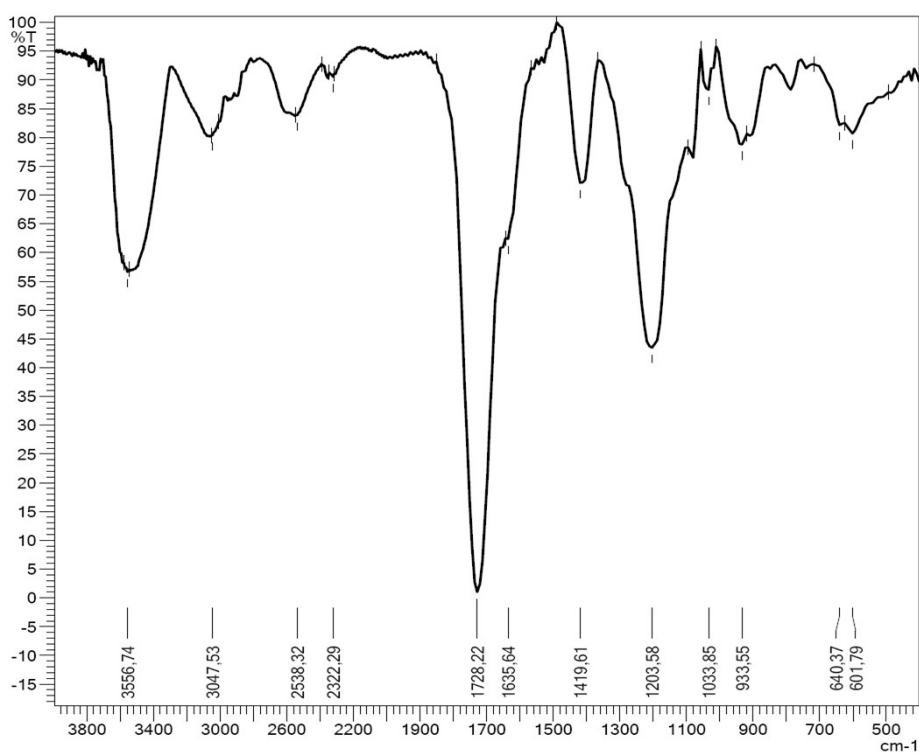
FT-IR spectrum of the Bio-oil recovered after 3 hours at 155 °C.
