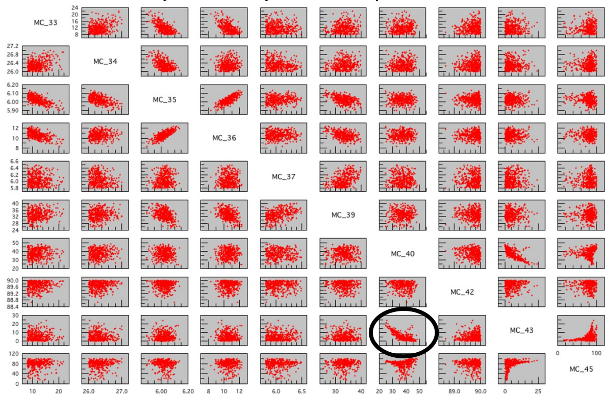
Figure S6. Monte Carlo error analysis showing correlation between the thickness of the 4 th and the 5 th layer (indicated with a black circle).
