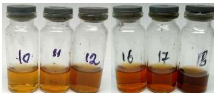
Fig. S3. Stability of AgNPs in six month after the initiation by Artemisia tilesii “hairy” root extracts
