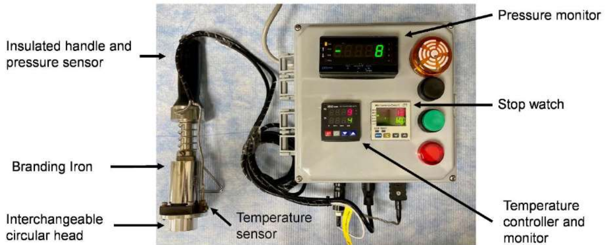
Figure S1. Custom burn wound device. Features of the device that regulate delivery of thermal energy and pressure to create consistent burn wounds. Plans are available upon request.
