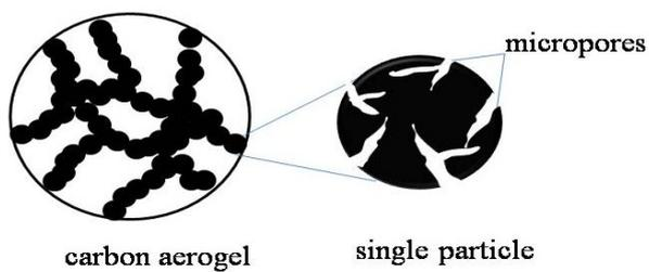
**Fig. S5.** Formation of micropores by skeleton particles
