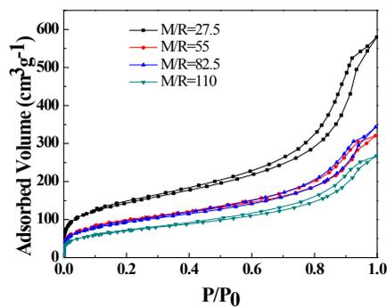
**Fig. S2.** The nitrogen adsorption isotherms of the RF aerogels synthesized by various M/R ratios. The Z/R ratio is kept constant as 6.48.
