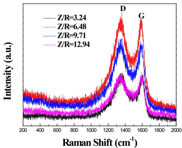
**Fig. S6.** Raman spectra of carbon aerogels synthesized by various Z/R ratios
