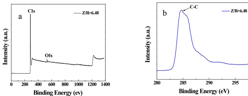
**Fig. S9.** Broad XPS spectra (a) and C 1s spectra (b) of as-prepared carbon aerogel
