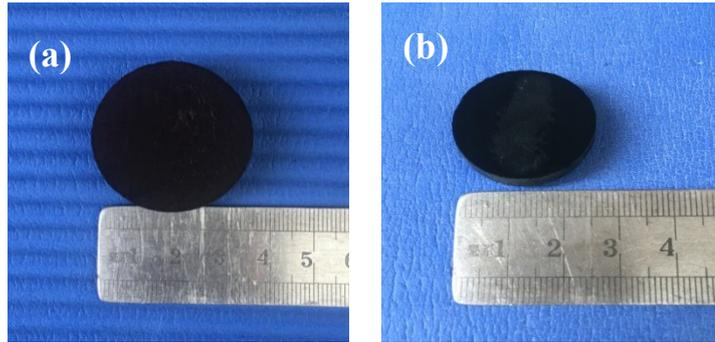
**Fig. S1.** Photos of RF aerogel (a) and derived carbon aerogel (b) synthesized by salt template
