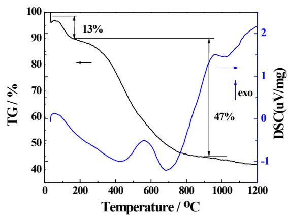
**Fig. S10.** TG-DSC curves of RF aerogel in argon atmosphere
