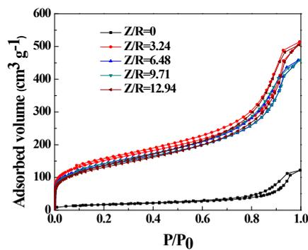
**Fig. S3.** The nitrogen adsorption isotherms of RF aerogels synthesized by various Z/R ratios. The M/R ratio is kept constant as 40.
