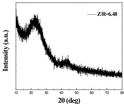
**Fig. S7.** XRD pattern of carbon aerogel synthesized by salt template
