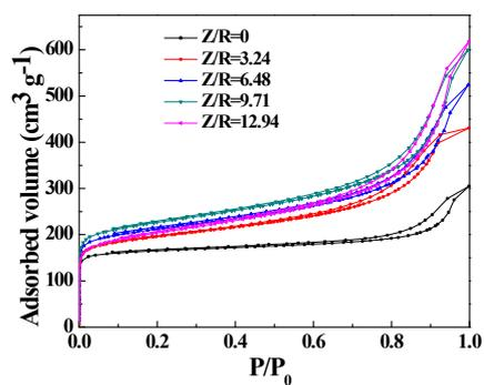
**Fig. S4.** The nitrogen sorption isotherms of carbon aerogels synthesized by various Z/R ratios. The M/R ratio is kept constant as 40.
