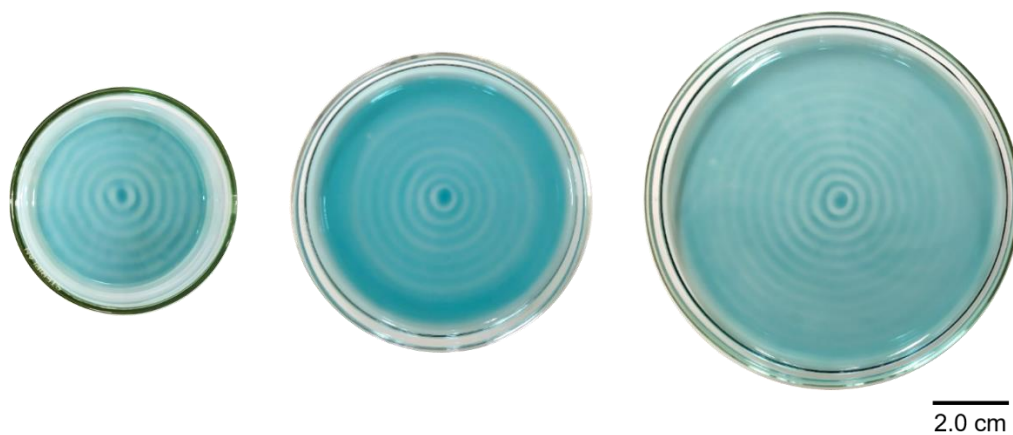
Supplementary Figure 5. Cascade reactions within transient domains in a solution obtained with different sized Petri dishes. Pattern images of glucose/GOx/HRP/ABTS cascade reaction system obtained with different sized Petri dishes by applying 30 Hz of audible sound. The inner diameter of the dishes is 56, 76, and 96 mm in size, respectively.
