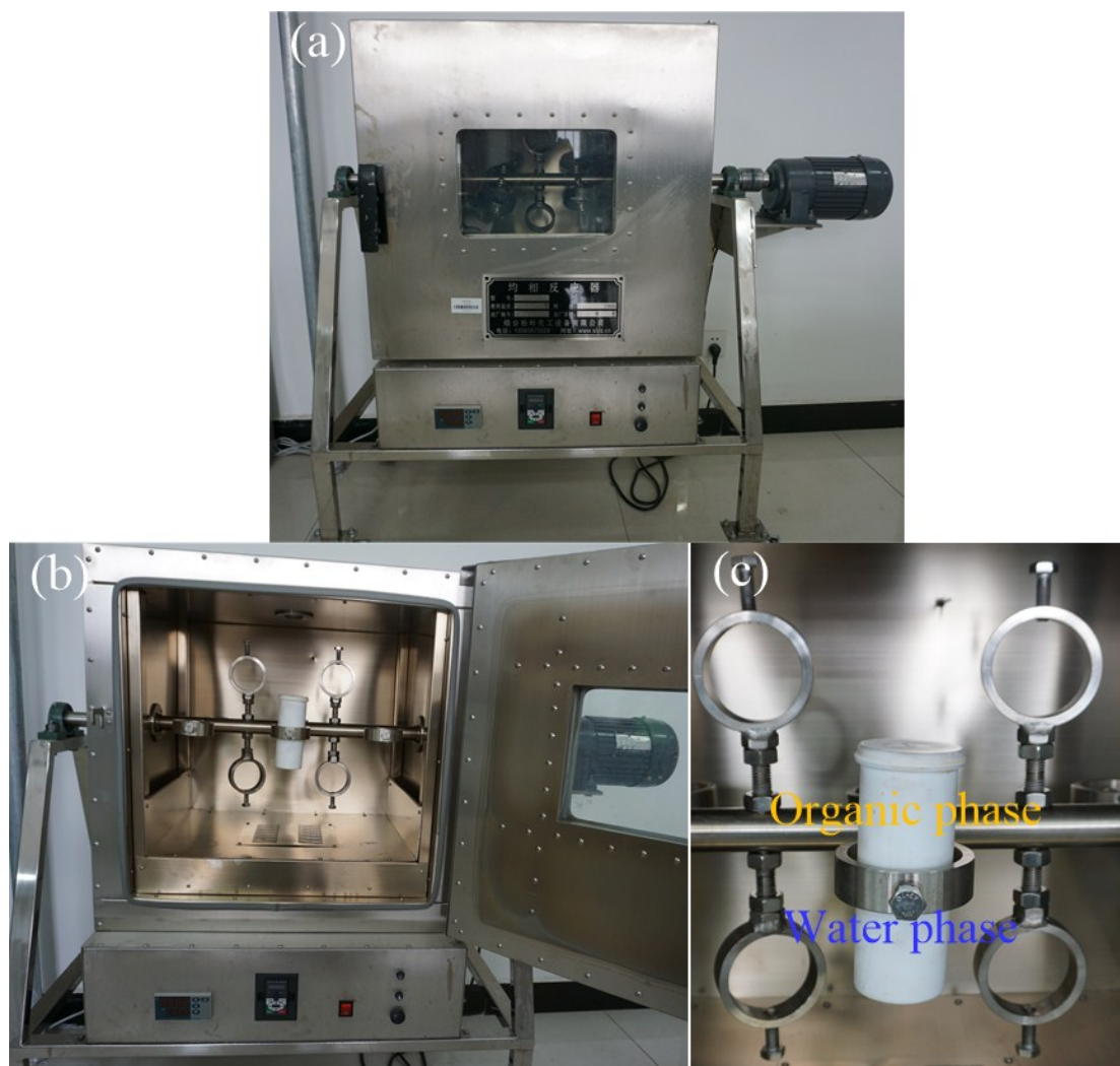
Fig. S3 A one-pot rotating hydrothermal system for KCC-1 fabrication. Organic phase mainly is cyclohexane (See synthesis process of experimental details).
