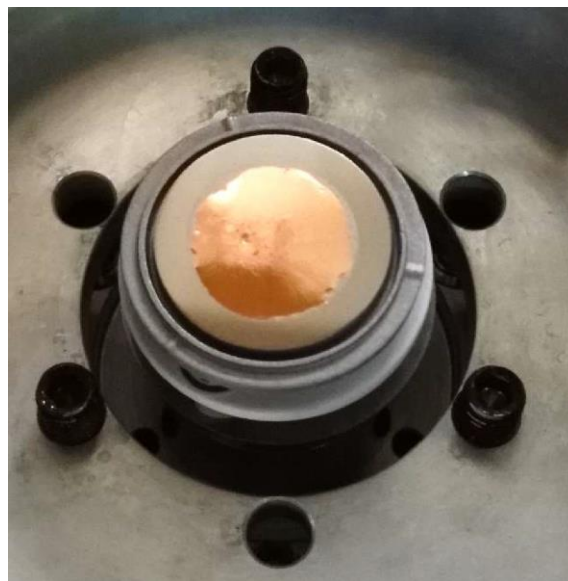
Figure S1 Photo of the copper surface on the tungsten disk and heater after the melting and solidification of a 40 \mu\text{m} -thick copper foil. The diameter of the copper dome is about 10 mm.
