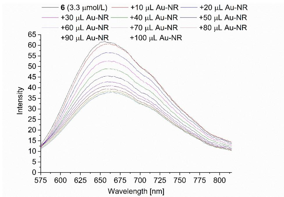
**Figure S26** Fluorescence spectra of PD **6** ( $c = 3 \mu\text{mol/L}$ ) with the stepwise addition of 100  $\mu\text{L}$  Au-NR dispersion (excitation wavelength = 470 nm).
