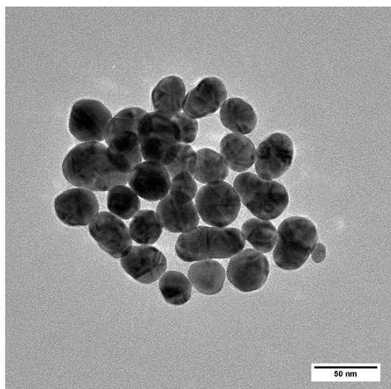
**Figure S4** TEM images of the synthesized Au-NPs after the addition of acetone (to a 1:1 v:v mixture) to the of aqueous Au-NP dispersion.
