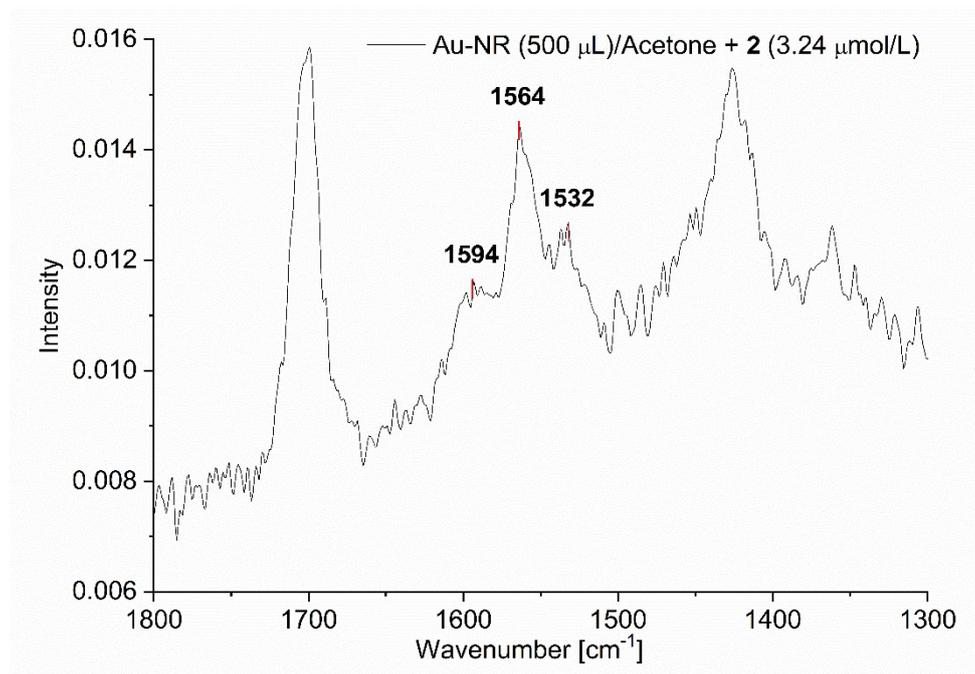
**Figure S20** SERS studies (200 mW) for PD 2@Au-NR at 3.24 μmol/L in H<sub>2</sub>O/acetone (1:1 v:v) (section between 1800-1300 cm<sup>-1</sup>).
