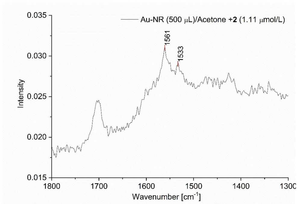
**Figure S21** SERS studies (200 mW) for PD **2**@Au-NR at 1.11 μmol/L in H<sub>2</sub>O/acetone (1:1 v:v) (section between 1800-1300 cm<sup>-1</sup>).
