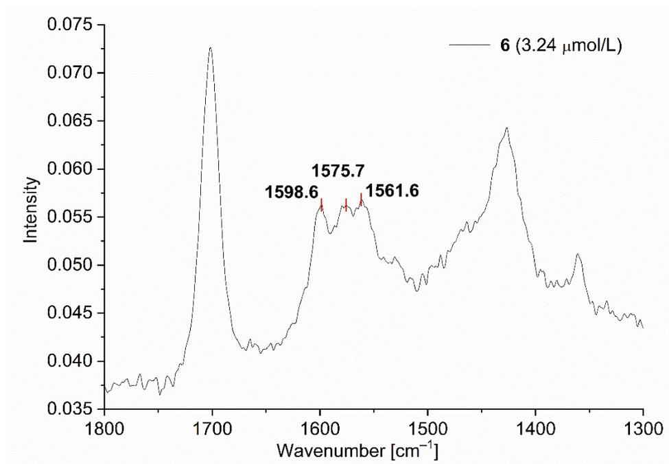
**Figure S11** SERS studies for PD 6@Au-NP at 3.24 μmol/L (500mW) in H<sub>2</sub>O/acetone (1:1 v:v) + 10 mg KCl added to 3 mL of the dispersion.
