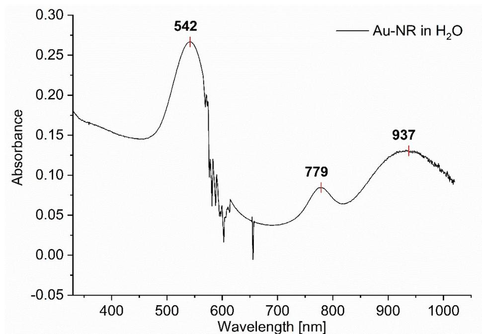
**Figure S6** UV/Vis spectrum of Au-NR/water dispersion. The peak at 542 nm refers to the transverse axis, the peak at 937 nm a peak to the longitudinal axis. At 779 nm a small peak for gold nanoprisms occurred (see Fig. S5), where the reaction was not completed to nanorods.
