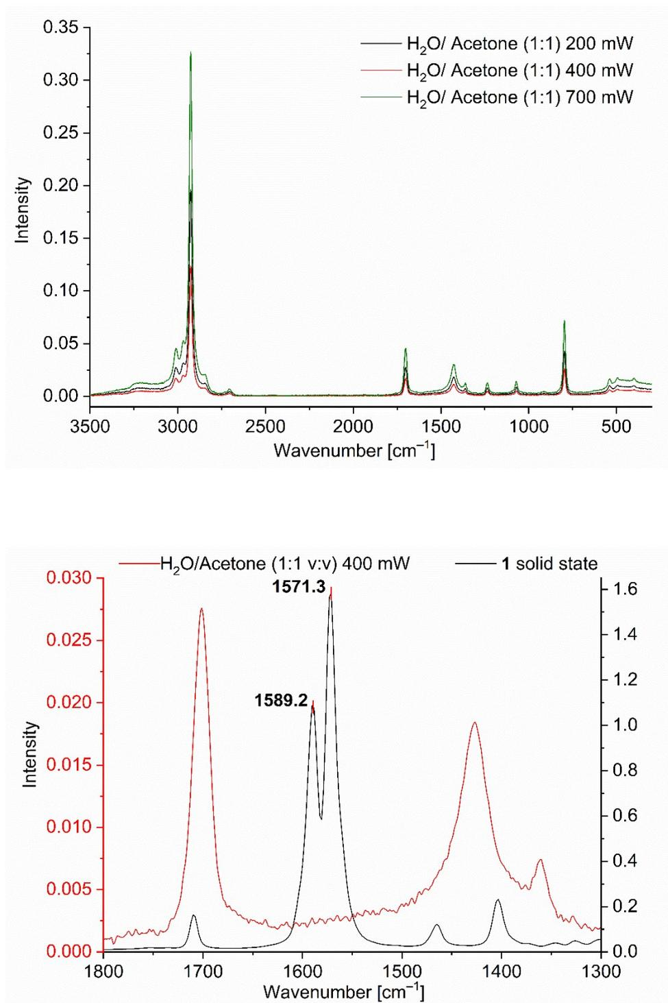
**Figure S7 Top** Raman spectrum of an H<sub>2</sub>O/acetone (1:1 v:v) mixture at 200, 400, 700 mW Laser output. **Bottom** Comparative overlay of the Raman spectrum of PD 1 (solid state, black) and of the H<sub>2</sub>O/acetone (1:1 v:v) mixture in the spectral region between 1800-1300 cm<sup>-1</sup>
