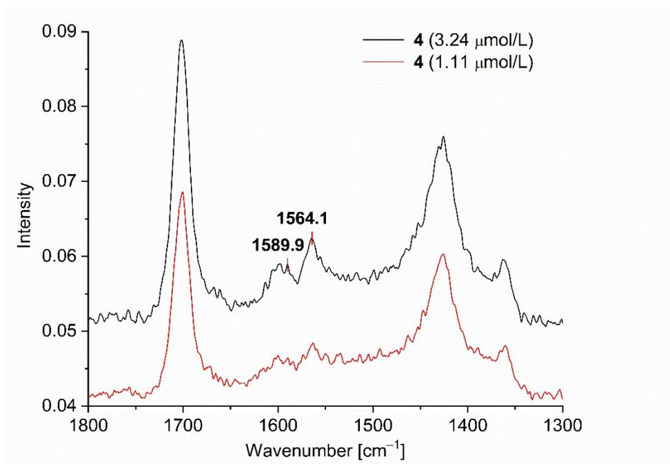
**Figure S10** SERS studies for PD 4@Au-NP at 3.24 (500 mW), 1.11 (700 mW) μmol/L in H<sub>2</sub>O/acetone (1:1 v:v) + 10 mg KCl added to 3 mL of the dispersion.
