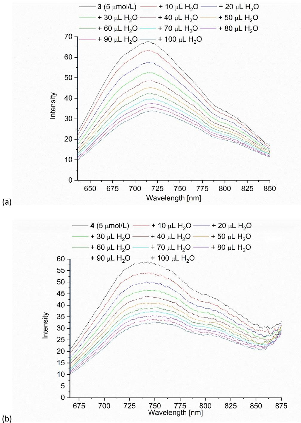
**Figure S16 a)-b)** Fluorescence spectra of PD **3** and **4** ( $c = 5 \mu\text{mol/L}$ ) with the stepwise addition of  $100 \mu\text{L H}_2\text{O}$  (excitation wavelength a)  $466 \text{ nm}$  b)  $494 \text{ nm}$ ). Concentrations were higher than for PD **1** and **2** and **5** and **6** due to lower fluorescence intensities.
