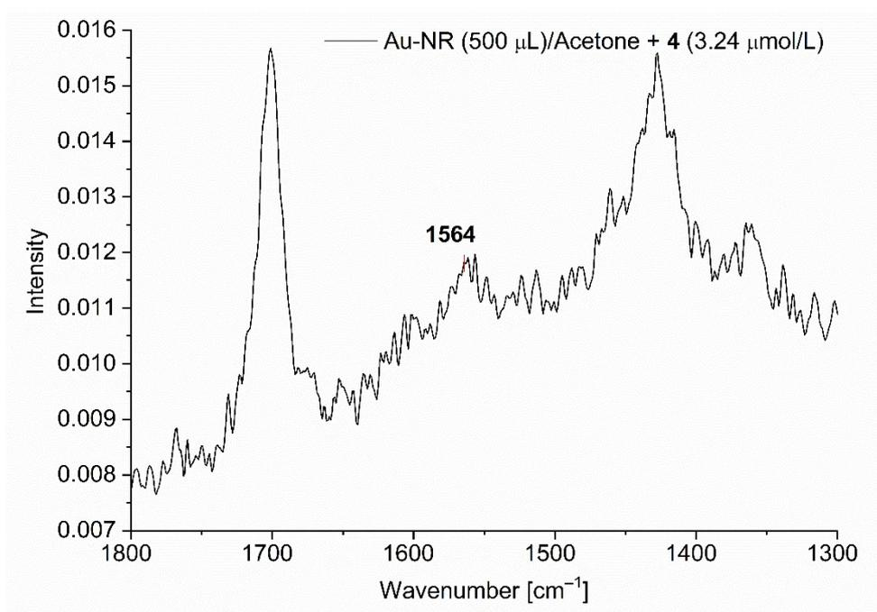
**Figure S22** SERS studies (200 mW) for PD **4**@Au-NR at 3.24 μmol/L in H<sub>2</sub>O/acetone (1:1 v:v) (section between 1800-1300 cm<sup>-1</sup>).
