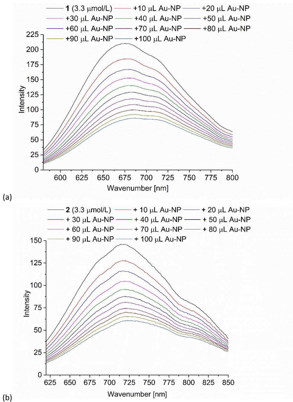
**Figure S12 a)-b)** Fluorescence spectra of PD 1 and PD 2 ( $c = 3.3 \mu\text{mol/L}$ ) with the stepwise addition of 100  $\mu\text{L}$  Au-NP dispersion (excitation wavelength a) 450 nm b) 465 nm).
