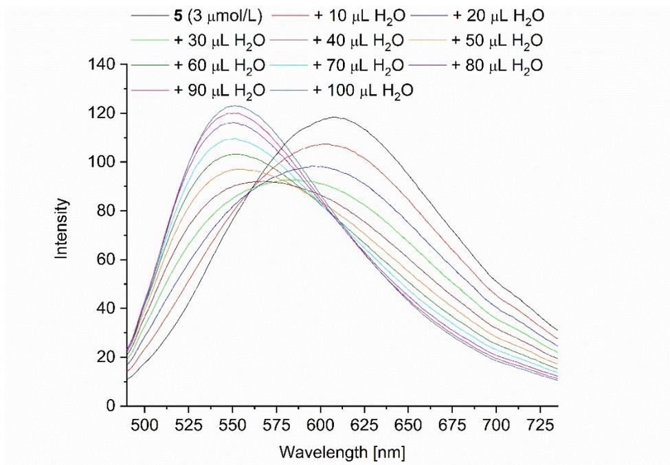
**Figure S17** Fluorescence spectra of PD 5 ( $c = 3.3 \mu\text{mol/L}$ ) with the stepwise addition of 100  $\mu\text{L H}_2\text{O}$  (excitation wavelength = 428 nm).
