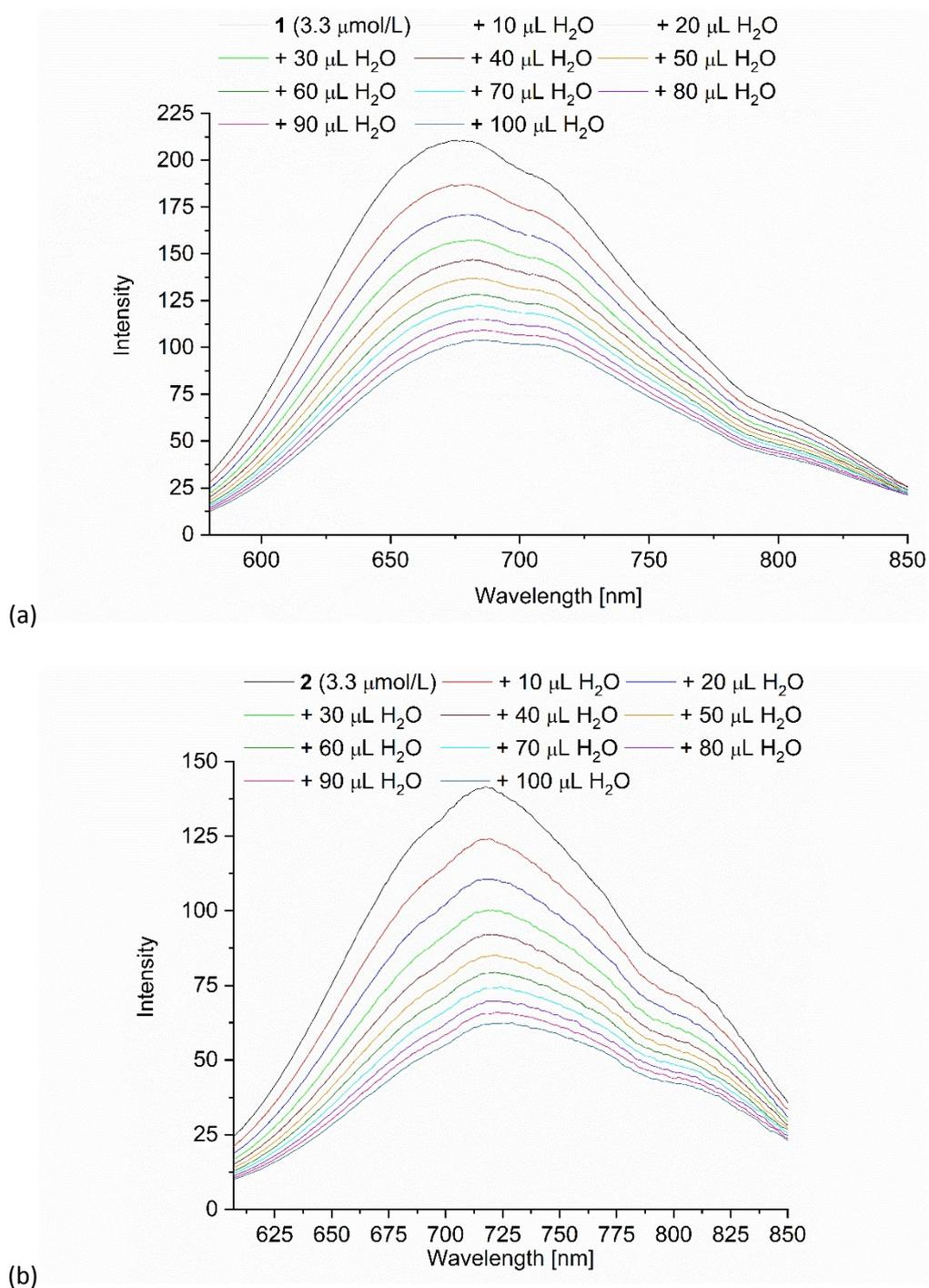
**Figure S15 a)-b)** Fluorescence spectra of PD 1 and PD 2 ( $c = 3.3 \mu\text{mol/L}$ ) with the stepwise addition of 100  $\mu\text{L H}_2\text{O}$  (excitation wavelength a) 450 nm b) 465 nm).
