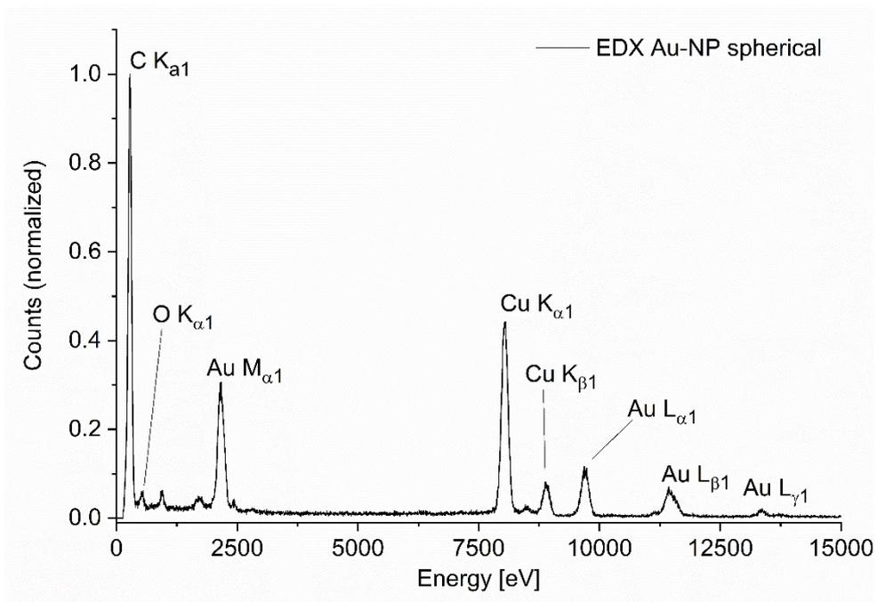
Figure S2 EDX spectrum of synthesized Au-NPs
