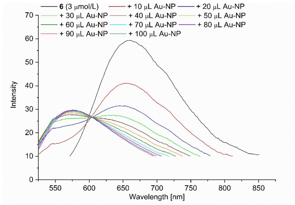
**Figure S14** Fluorescence spectra of PD **6** ( $c = 3 \mu\text{mol/L}$ ) with the stepwise addition of 100  $\mu\text{L}$  Au-NP dispersion (excitation wavelength = 470 nm).
