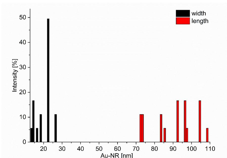
**Figure S5** TEM images and size histogram of the synthesized Au-NRs. TEM images show nanorods from three different spots on the TEM grid. The size of 18 particles was measured by hand.
