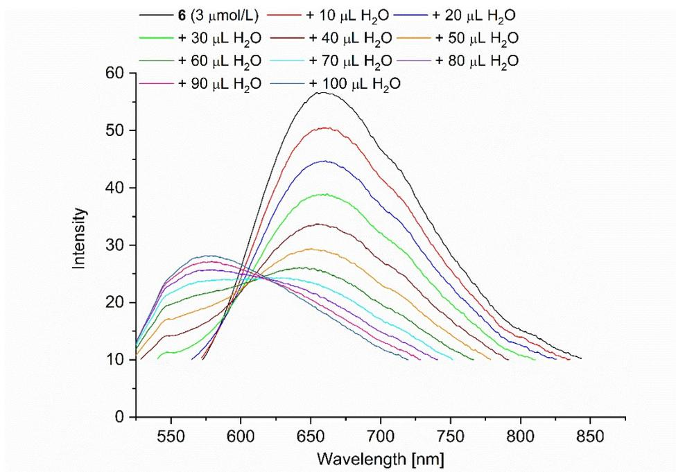
**Figure S18** Fluorescence spectra of PD 6 ( $c = 3 \mu\text{mol/L}$ ) with the stepwise addition of 100  $\mu\text{L H}_2\text{O}$  (excitation wavelength = 470 nm).
