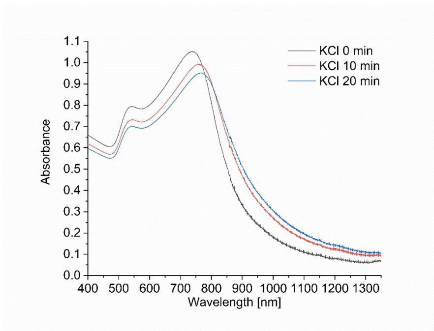
**Figure S3 Top** UV/vis spectrum of Au-NP/water dispersion. The band at 525 nm corresponds to the localized surface plasmon resonance (LSPR) band of the spherical gold nanoparticles <sup>[3]</sup>. **Bottom** Time dependent UV/vis/NIR absorption of Au-NPs in water/acetone (1:1 v:v) with KCl added.
