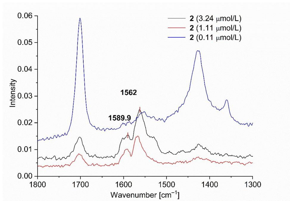
**Figure S8** SERS studies (200 mW) for PD **2**@Au-NP at 3.24, 1.11 (both 200 mW) and 0.11 μmol/L (700 mW) in H<sub>2</sub>O/acetone (1:1 v:v) + 10 mg KCl added to 3 mL of the dispersion.
