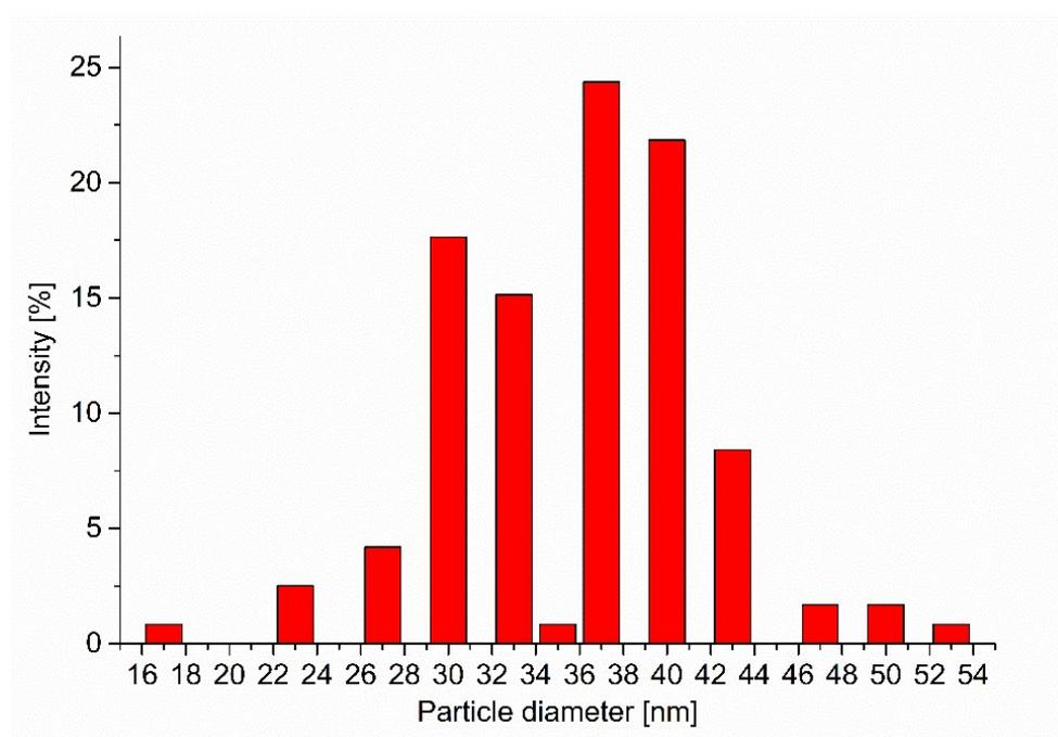
**Figure S1** TEM images and size histogram of the synthesized Au-NPs. The size of 119 particles was measured by hand.
