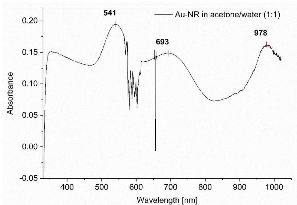
**Figure S19** UV/Vis spectrum of Au-NRs in water/acetone (1:1 v:v)
