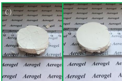
**Figure S3.** Photographs of PSA-7 after 70% compression. Few cracks were observed at the edge and surface (Left graph) of sample after compression. Bottom of the sample can remain smooth (Right graph).
