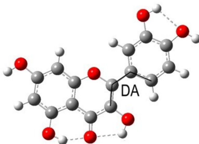
Figure S1. Quercetin fully optimized geometry, with a dihedral angle, DA, 21.63^\circ , according with Álvarez-Diduk et al. [3], where the colours code is: gray for carbon, red for oxygen and white for hydrogen atoms.
