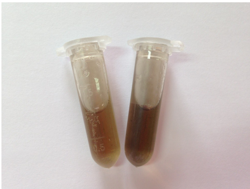
Fig. S1 Digital photograph of GO (left) and prGO (right) solution with the same concentration of 0.2 \text{ mg mL}^{-1} .
