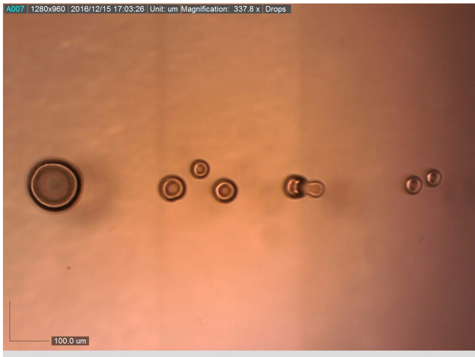
Figure S14: Substrate with large medium and small droplets with a platengap of 6.8 mm
