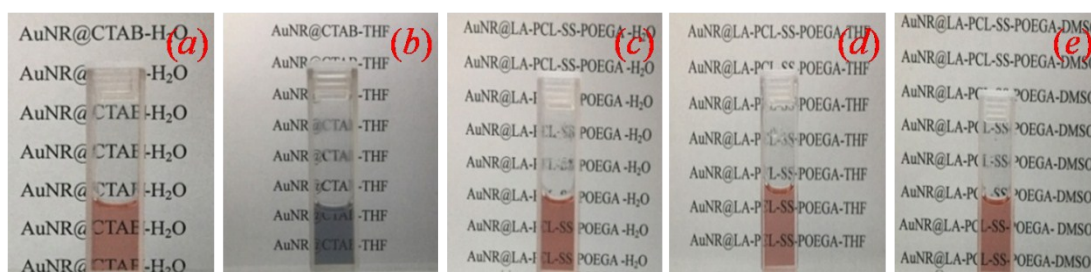
Figure S9. The images of AuNRs@CTAB dispersed in (a) \text{H}_2\text{O} and (b) THF, and AuNRs@LA-PCL-SS-POEGA dispersed in (c) water, (d) THF, and (e) DMSO.
