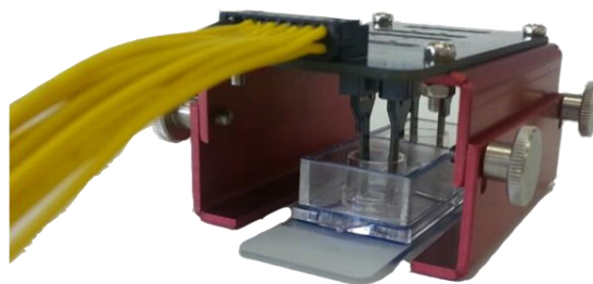
Fig. S1. Photos of the 2D and 3D impedance sensors. Photos of A) the 2D impedance cell sensor array consisting of 16 sensors and B) the 3D impedance cell sensor.
