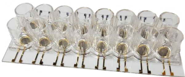
Fig. S1. Photos of the 2D and 3D impedance sensors. Photos of A) the 2D impedance cell sensor array consisting of 16 sensors and B) the 3D impedance cell sensor.
