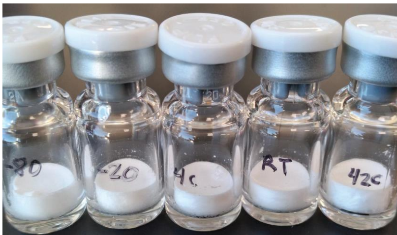
Figure S1. Related to Figure 1. Representative images of lyophilized vials containing Luc mRNA-LNPs. Luc mRNA-LNPs were stored at -80^{\circ}\text{C} , -20^{\circ}\text{C} , 4^{\circ}\text{C} , room temperature (RT, 25^{\circ}\text{C} ) or 42^{\circ}\text{C} for 0, 4 or 24 weeks. All lyophilized mRNA-LNPs formed a uniform, dense, white cake.
