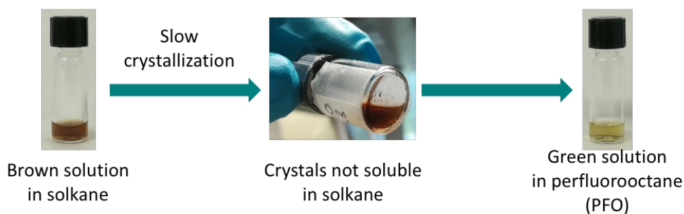
Supplementary Figure 5: Images of crude product in solkane, crystal formation and crystal solution in PFO.
