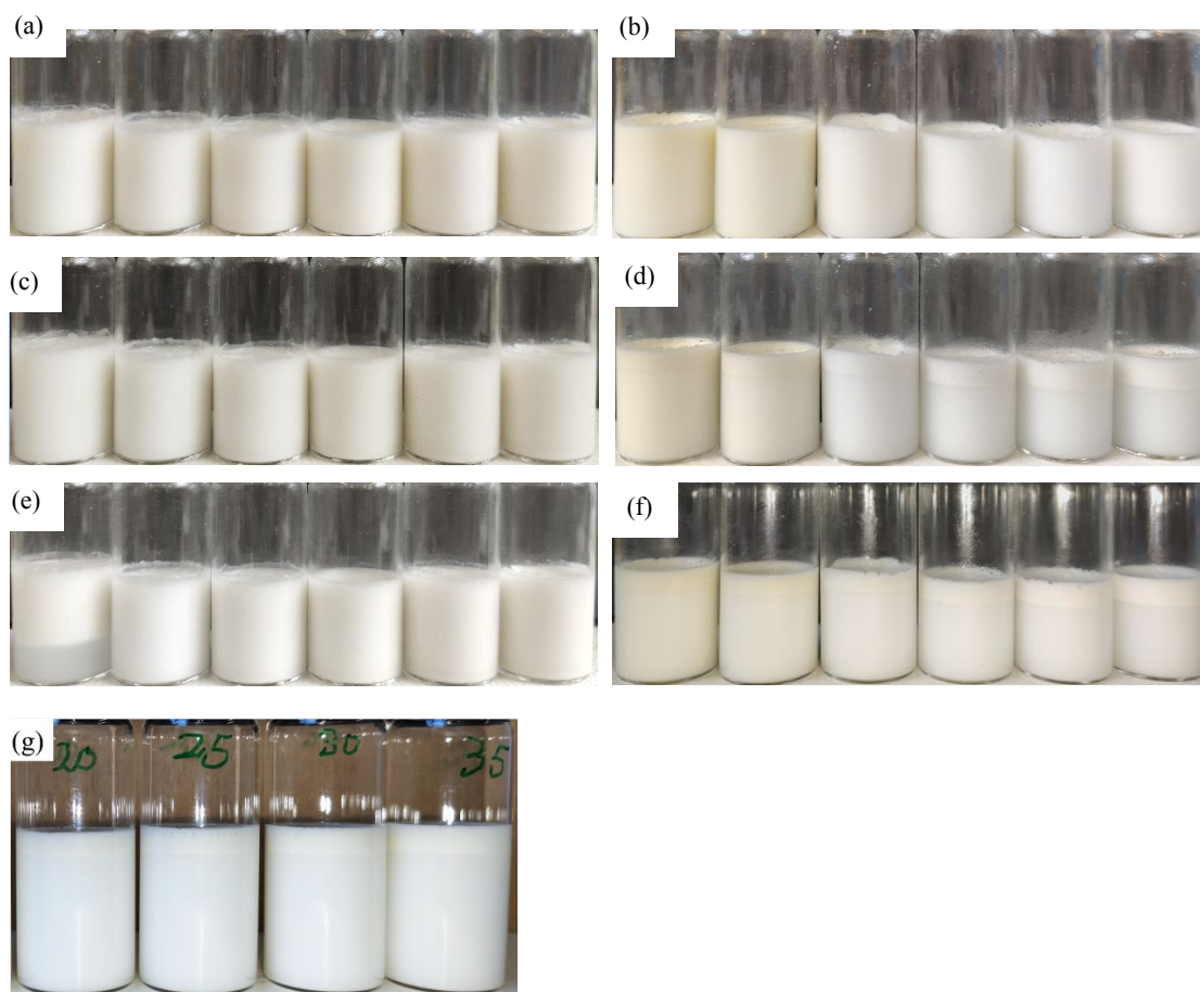
Figure S4. Linseed oil in water emulsions stored at room temperature (a) 10%~35% octyl-CNC stabilized emulsions right after sonication (b) 10%~35% sCNC stabilized emulsions right after sonication (c) 10%~35% octyl-CNC stabilized emulsions 1 hour after sonication (d) 10%~35% sCNC stabilized emulsions 1 hour after sonication (e) 10%~35% octyl-CNC stabilized emulsions 24 hours after sonication (f) 10%~35% sCNC stabilized emulsions 24 hours after sonication (g) 20%~35% sodium dodecyl sulfate stabilised emulsions 10 minutes after sonication.
