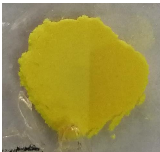
Supplementary Figure 18. The color changes of H 2 ADC after Xe lamp light irradiation.
