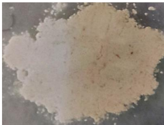
Supplementary Figure 8. The color changes of powder sample 1 after Xe lamp light irradiation.
