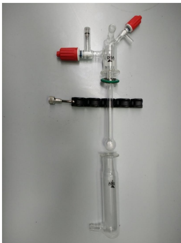
Figure S1. Picture of the cell employed for isothermal volumetric adsorption measurements. Italian patent application n°10202000005014 filed on March 9 th , 2020 and PCT n. PCT/IB2021/051769 filed on March 3 rd , 2021.
