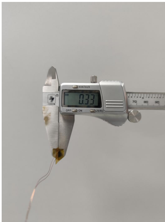
Figure S29. Optical image of the encapsulated PI/FCNT (EPD) pressure sensor. The thickness is 0.33 mm.
