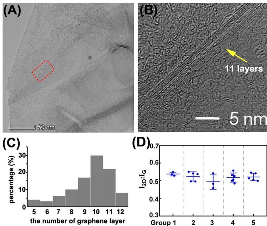
**Figure S2.** Characterization of graphene layers. A) TEM characterization of graphene layers. B) A magnified edge image obtained from the square-marked area of graphene sheet in panel A. C) The quantification of the number of CVD-synthesized graphene layers. D) Ratio of the Raman 2D- and G-peaks in graphene of different group.
