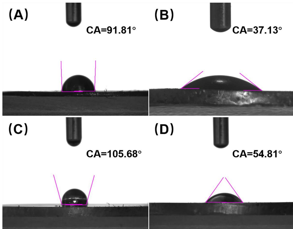
**Figure S3.** Hydrophilicity of OP-treated graphene. The contact angle images of the A) surface of raw Graphene/PDMS, B) surface of OP-treated Graphene/PDMS, C) surface of PDMS, and D) surface of OP-treated PDMS.
