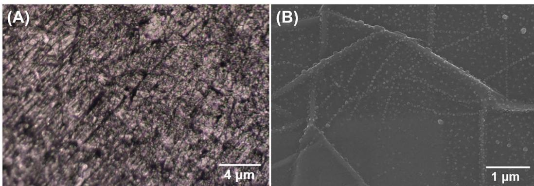
**Figure S1.** A) Raman image of the substrate (the surface of graphene). B) SEM image of the graphene surface.
