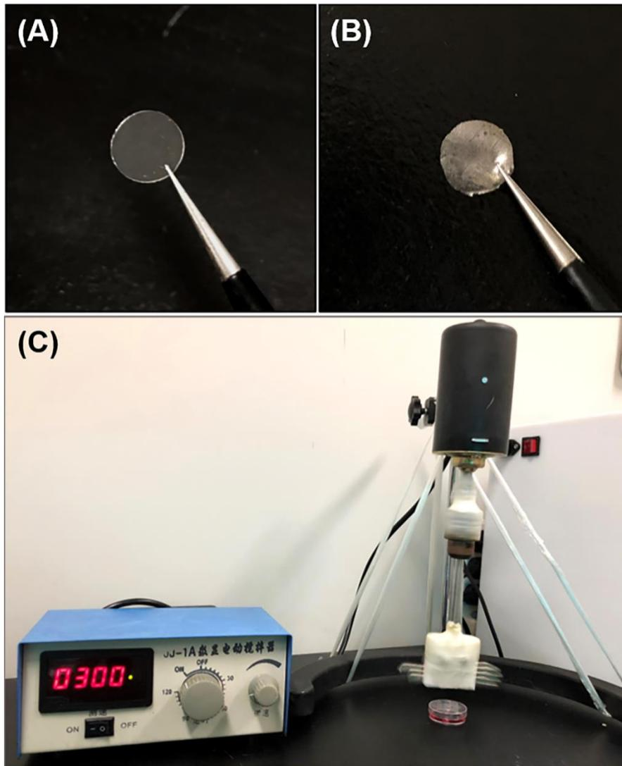
**Experimental substrates and equipment.** A) and B) The pictures of PDMS and graphene/PDMS substrates used in the experiment. C) The magnetic rotating equipment in the study.
