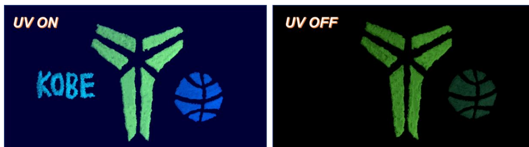
Fig. S10 Application of multiple anti-counterfeiting: the name of “KOBE” was written by pyrene—a conventional dimer fluorescent material; “Mamba” logo was written by 2PtzO-7C powder—pure dimer phosphorescence material and “basketball” written by 2PtzO-6C powder—dual phosphorescence emissions material (left: under 365 nm UV lamp; right: after the removal of 365 nm UV excitation). A very meaningful moral: Kobe is dead, but Mamba Mentality and basketball faith are forever.
