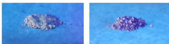
Figure S1. Photograph of the Tb 3+ solution-immersed ground raw materials before and after the acid treatment (left to right).
