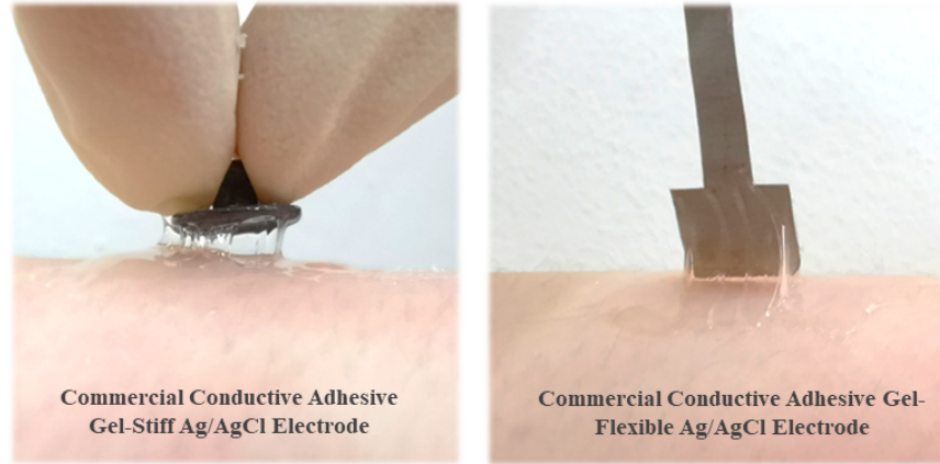
Fig. S4. Inferior mechanical interaction of commercial EEG gel with electrodes. Photographs of detached stiff and flexible Ag/AgCl electrodes from the commercial EEG adhesive gel on the skin when pulling these electrodes.
