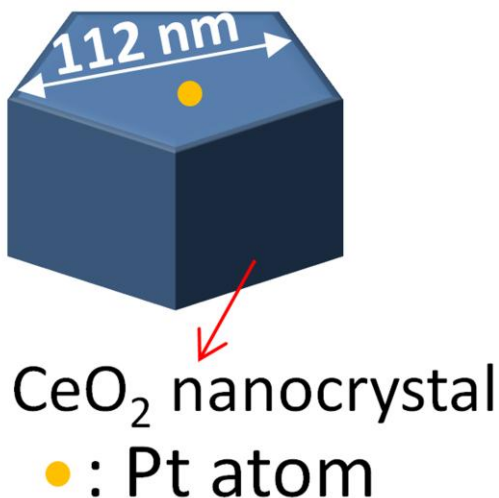
Scheme S1 The loading of single Pt atom on single CeO_2 nanocrystal with size of about 112 nm for the calculation of Pt content.
