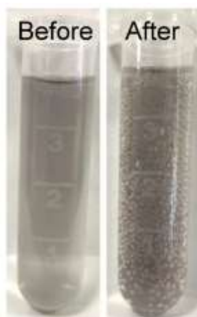
Figure S10. O 2 generation photographs of MO@FHO before and after adding H 2 O 2 . The 4 mL of MO@FHO solution (0.05 mg mL -1 in deionized water) is placed in a centrifuge tube, and subsequently adding 40 μL of H 2 O 2 solution (1 M in deionized water).
