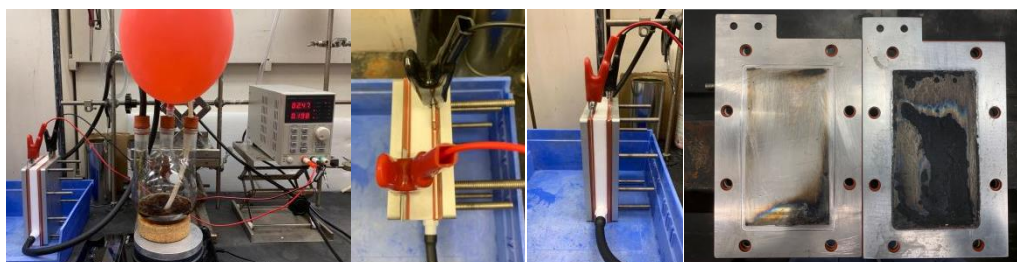
Left to right: 100g scale in recycle flow; top view of cell; side view of cell; cathode/anode after reaction.
