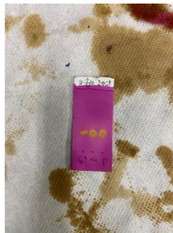
Left: Reaction mixture was diluted with Et 2 O and filtered through a thin layer of silica. Center: Removal of solvent. Right: Crude TLC (20:1 Hexanes: EA).
