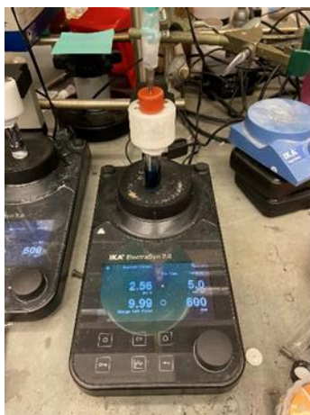
Left: Start the reaction with a stirring speed of 600 rpm. Center: Reaction completed. Right: Electrodes were rinsed with Et 2 O and transferred into a separatory funnel.
