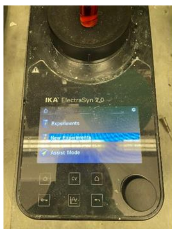
Left: Select 'New Experiments'. Center: Select 'Constant Current'. Right: Set the current to 5 mA.
