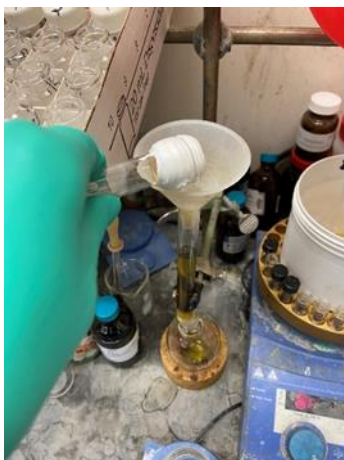
Left: Reaction mixture was diluted with Et 2 O and filtered through a thin layer of silica. Center: Removal of solvent. Right: Crude TLC (20:1 Hexanes: EA).
