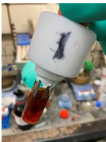
Left: The cap was tightly screwed into the vial. Center: Purging with Argon for 5 min. Right: The electrochemical cell was plugged into ElectraSyn 2.0.
