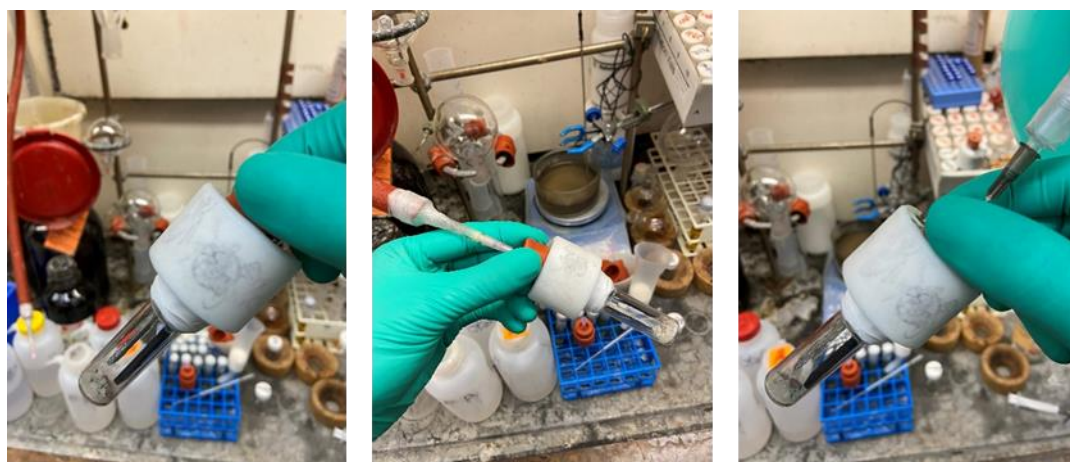
Left: \text{CoBr}_2 .glyme (6.2 mg). Center: 6,6-Me 2 -bpy (5.5 mg). Right: \text{Et}_3\text{NHBF}_4 (114 mg).
