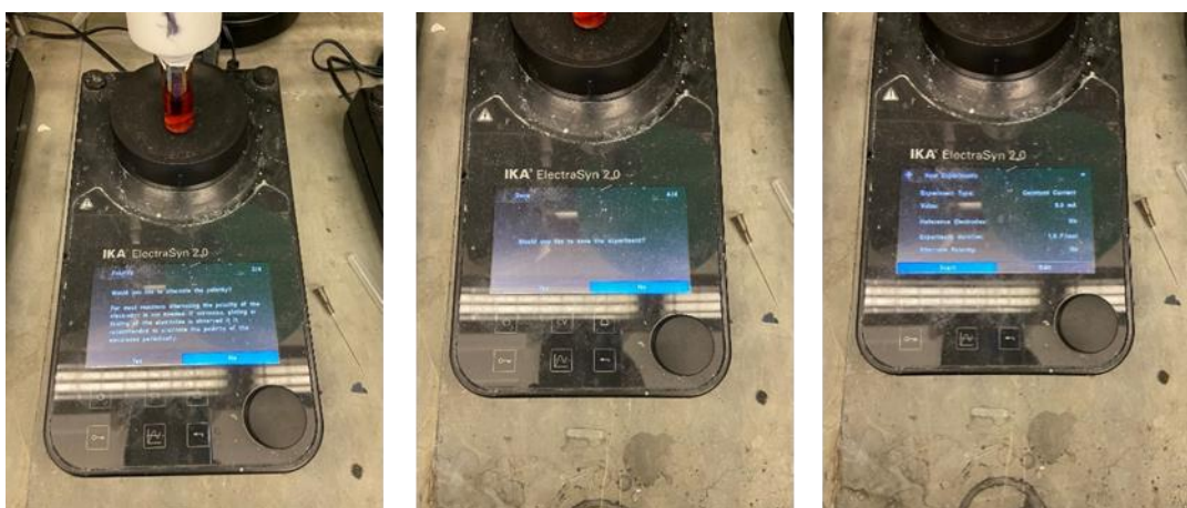
Left: No alternate polarity. Center: Saving the experimental parameters is optional. Right: ElectroSyn is ready.
