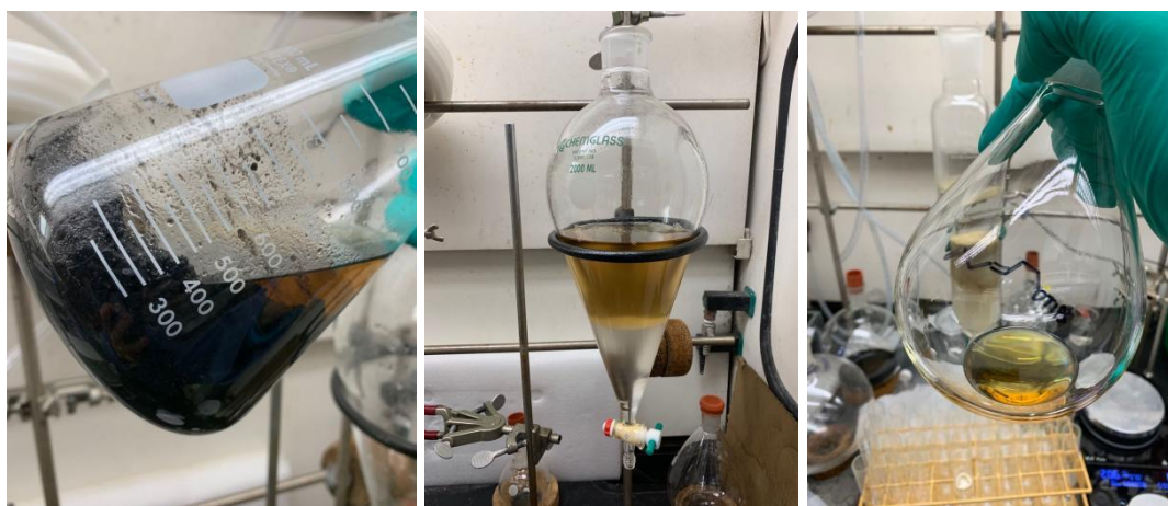
Left to right: Rochelle salt wash reaction crude; brine wash in separatory funnel; column chromatography and isolated product.
