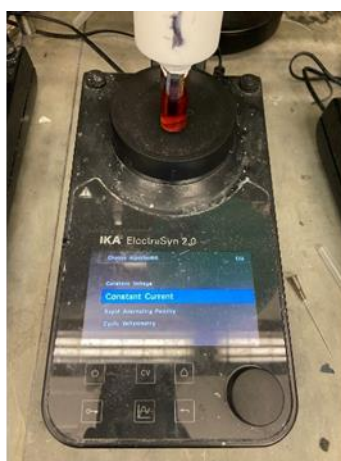
Left: Select 'New Experiments'. Center: Select 'Constant Current'. Right: Set the current to 5 mA.
