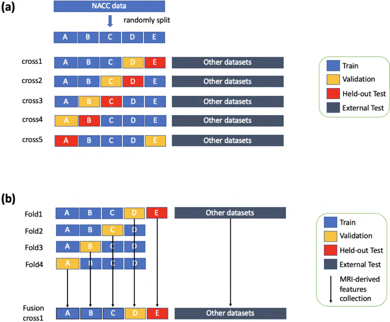
Supplementary Figure S12: Data splitting strategy. (a) A schematic showing the data splitting strategy used for training, validation, and testing of the model is shown. NACC data was split into five folds (labeled A-E) for cross-validation, each of which was enforced to have identical class ratios of NC, MCI, and DE cases. In each cross-validation experiment, different portions of NACC were used for training and validation; all other datasets were kept for external testing. (b) A schematic is shown demonstrating how MRI-derived features were collected for usage in a fusion model. The MRI-derived features used in the fusion model were the direct outcomes from the multi-task CNN model, i.e., raw output from the COG task (i.e., DEMO score) and ALZ score from the AD classification task. To avoid information leakage, we did not collect MRI-derived features from the training part. Instead, we only collected MRI-derived features either from the validation set or the testing set. To collect MRI-derived features from all cases, we shuffled the training and validation parts for four times as illustrated.
