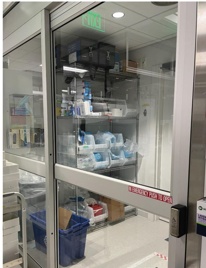
Supplemental Figure 1 The entrance to the laboratory was modified with the installation of an automated sliding door to separate the main laboratory space from the entryway. The image shows a gowning area for laboratory staff to put on appropriate personal protective equipment. Personal protective equipment shown in this space includes gloves, lab gowns, isolation lab gowns, booties, and face shields. This image is taken from inside the laboratory looking into the Lab Entryway labeled in Figure 2b .
