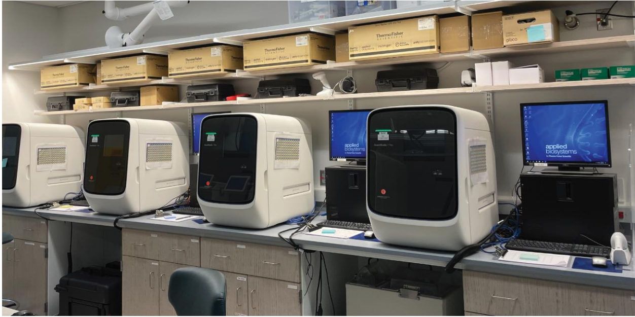
Supplemental Figure 4 The last step of the process is RT-qPCR which are run on 1 of 4 PCR machines located on the RT-qPCR section of the laboratory ( Fig. 2b ). Plates are manually loaded into the PCR machine after being prepared on the last robot.
