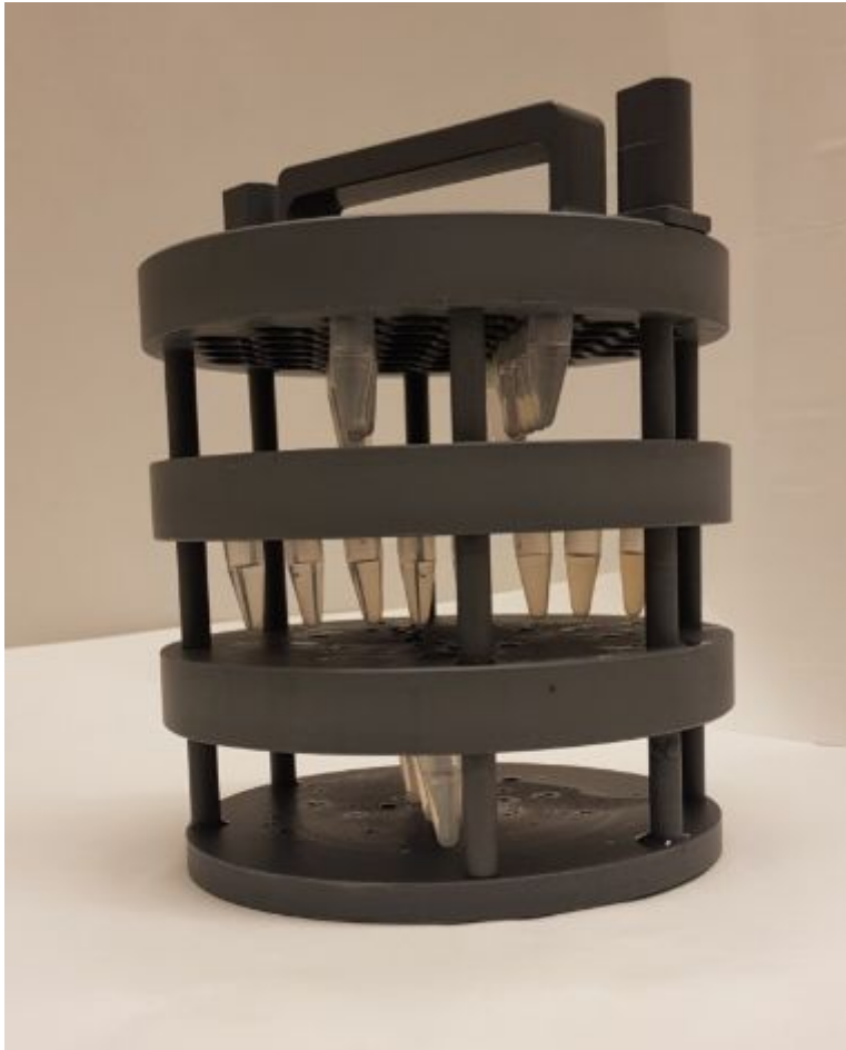
Figure S4. The three-level phantom model used in the MRI-experiments. Photograph courtesy of first author, P. Eriksson. Copyright 2020.
