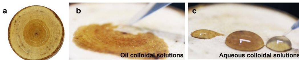
Supplementary Fig. 26. Dropping toluene and aqueous colloidal solutions on the wood surface. a, Photo of the wood before treatment. b, c, The toluene colloidal solution spread on the wood surface immediately, while it was difficult for the aqueous colloidal solution to spread on the wood.
