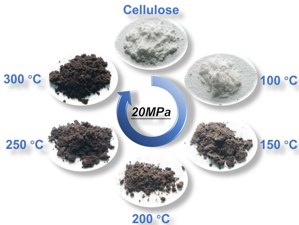
Supplementary Figure 16 | Macroscopic morphologies of hydrothermally treated cellulose from different stages (temperatures) of the hydrothermal reaction at 20 MPa.
