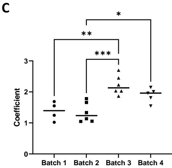
**Figure S3: Mechanical testing of milliPillar PDMS pillars. (A)** Force as a function of distance coefficients calculated using a microtester. **(B)** Representative force as a function of distance testing curve showing no apparent hysteresis of PDMS pillars. **(C)** Batch to batch variation among four batches of milliPillar platforms, n=4-6.
