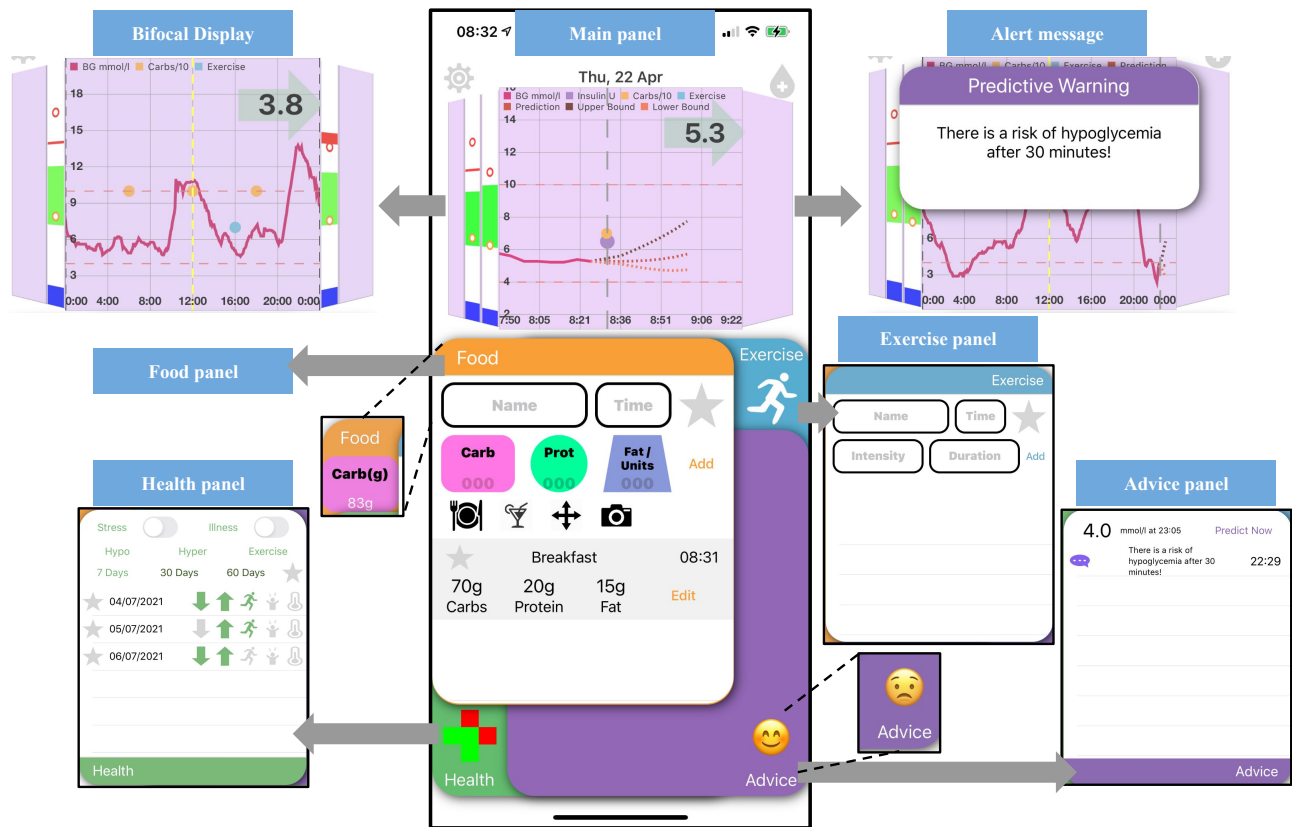
Supplementary Figure 1: Graphical user interface of the ARISES app, where bifocal display is used to present glucose trajectories. The users are allowed to record daily activities through the food, exercise and health panels. The embedded deep learning algorithm predicts glucose levels and detects hypo- and hyperglycemia with lower and upper bounds. Then the app sends corresponding warnings to users by notifications and haptic vibration and displays information in the advice panel. The corner icons of the food and advice panels can show the details of carbohydrate and the status of unread alert messages, respectively, when these panels are stacked at the bottom.
