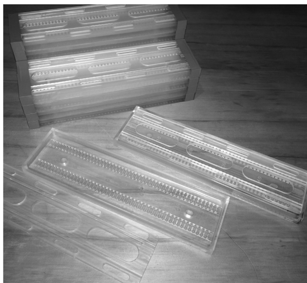
FIGURE 2 Plastic trays used to incubate wool fibers that had been mounted between plastic anchors in label and wash solution prior to stretching. The lower tray held the mounted hairs in an unstretched state, and the lid secured the anchors while allowing solutions access to the hairs.
