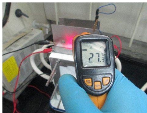
(Left) Frame cell and DC power during electrolysis. (Right) Temperature monitor of frame cell.
