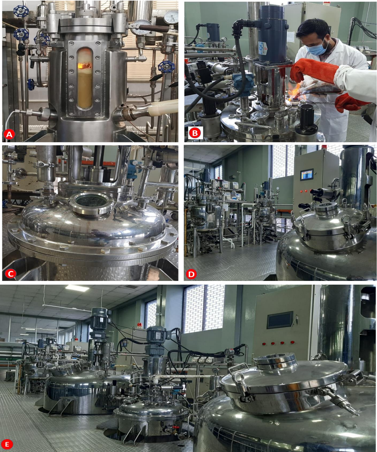
Supplementary Fig. F9: A) Laboratory Bioreactor: 10L. B) Seed culture vessel: 30L. C) Pilot Bioreactor: 300L. D. Industrial Bioreactor: 3000L. E) Fermentation floor.
